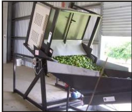
The fruit holding bin is placed into the lifting frame by forklift or pallet jack, the operator then uses a lever to raise the bin to a satisfactory position where a hand operated gate, which is adjusted prior to lifting, helps to regulate the flow of fruit.
